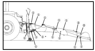
Figure 8 - Lubrication Points for Model 865H
